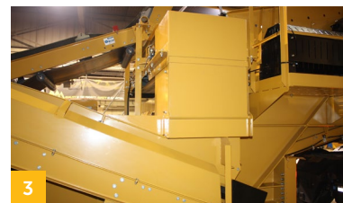
3 Ability to return top and middle deck oversized material back to the crusher. This feature increases production by splitting the load on two decks rather than one.
