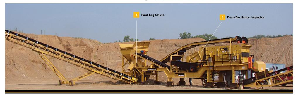
IROCK's Sidewinder reduces wear and increases production by screening out the sized material and crushing only oversized material. These secondary crushing plants come in three models and feature fast set-up, easy maintenance and extreme durability for a variety of crushing applications.
