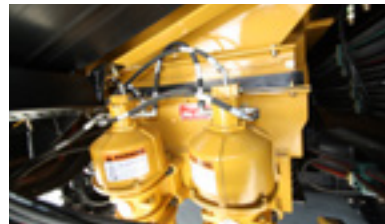
Optional vibrating crusher discharge pan feeder minimizes the risk of ripping the main conveyor belt in recycling applications. Stainless steel liners prevent material buildup in sticky applications.
