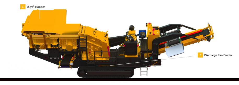
The TC-15 Mobile Open Circuit or Closed Circuit Horizontal Shaft Impact (HSI) Crusher designed for contractors with easy maneuverability, optimal versatility and high productivity. Its 15 yd<sup>3</sup> hopper allows you to feed material using a large wheel loader or excavator. And with the unit's 5' x 12' double deck screen and return conveyor that swings out to stockpile material, you can produce as many as four products or just one by simply closing the circuit.
