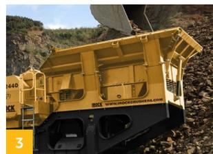
**3** Folding HARDOX® hopper mounted over vibrating feeder with optional integral pre-screen. Feeder rate can be regulated manually or automatically by loadsensing jaw.
