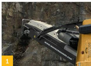
**1** Extended 42' main conveyor as standard, giving large stockpile capacity. Conveyor lowers and raises hydraulically.
