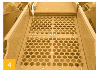
**4** Optional independent crusher pre-screen maximizes crusher efficiency and delivers screened product via side conveyor.
