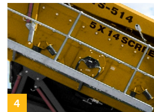
4 User friendly wedge system ensures faster screen changes.
