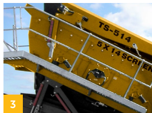
3 High Energy 14' x 5' (4200x1524mm) screenbox provides comparable product capacity with other larger class competitor's models.
