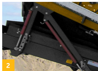
2 Hydraulic Screenbox linkage system, allows greater accessibility for screen change and enables optimum screen coverage at varying screenbox angles.
