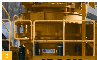
3 Dynamic adjust-closed side setting (CSS) can be changed while operating, minimizing downtime.
