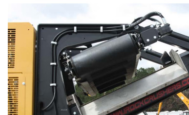
Reversible magnet enables material separation from the source material.
