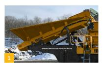
Heavy-duty steel hopper with adjustable feed rate via control panel, remote control or fully automatic regulation with feedback from the cone.
