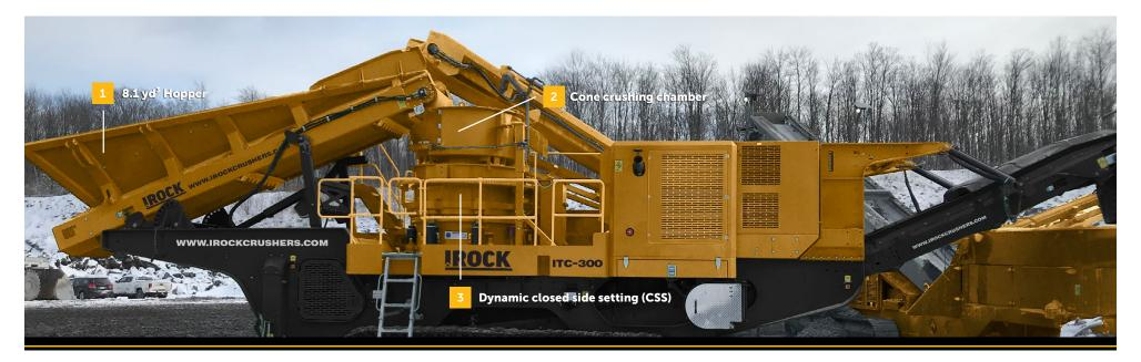
The IROCK ITC-300 Cone Crusher is known for proven performance with its 44" cone. Offering high material capacity and throughput, large stockpile capacity, and customer focused features. The ITC-300 provides a high degree of control over the final product, making it the ideal portable secondary crusher.
