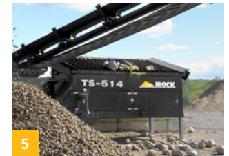
5 14' (4267mm) grid opening allows the use of larger loading shovels.
