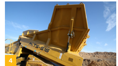
4 The heavy-duty, direct-feed system includes a rubber belt feeder and an optional HARDOX® apron feeder for increased longevity in rigorous applications.
