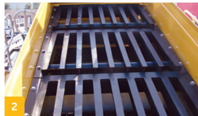
2 High-energy, two-bearing, 16' x 5' screen box, with 157ft² of screening area can sort up to three different product sizes. Optional top deck bofar bars, top deck punch plate, heavy-duty top finger deck and bottom finger deck.
