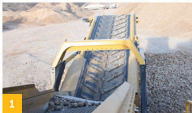
1 A 63" wide discharge conveyor, the widest in the industry, reduces jamming at the screen's discharge point.
