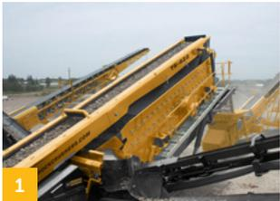
1 48" (1200mm) feed conveyor enables high capacity screening.
