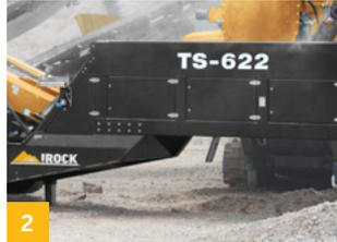
2 Up to 13.1 yd<sup>3</sup> (10m<sup>3</sup>) high capacity hopper with generous grid opening allows the use of larger loading shovels.
