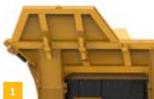
1 Folding HARDOX® hopper mounted over vibrating pan feeder with integral grizzly pre-screen. Feeder rate regulated manually or automatically by load sensing jaw.
