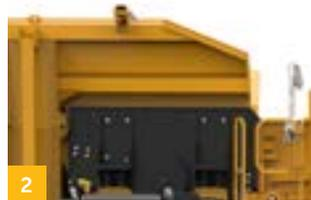
2 Optional independent crusher pre-screen feeder maximizes crusher efficiency and delivers screened product via side conveyor.
